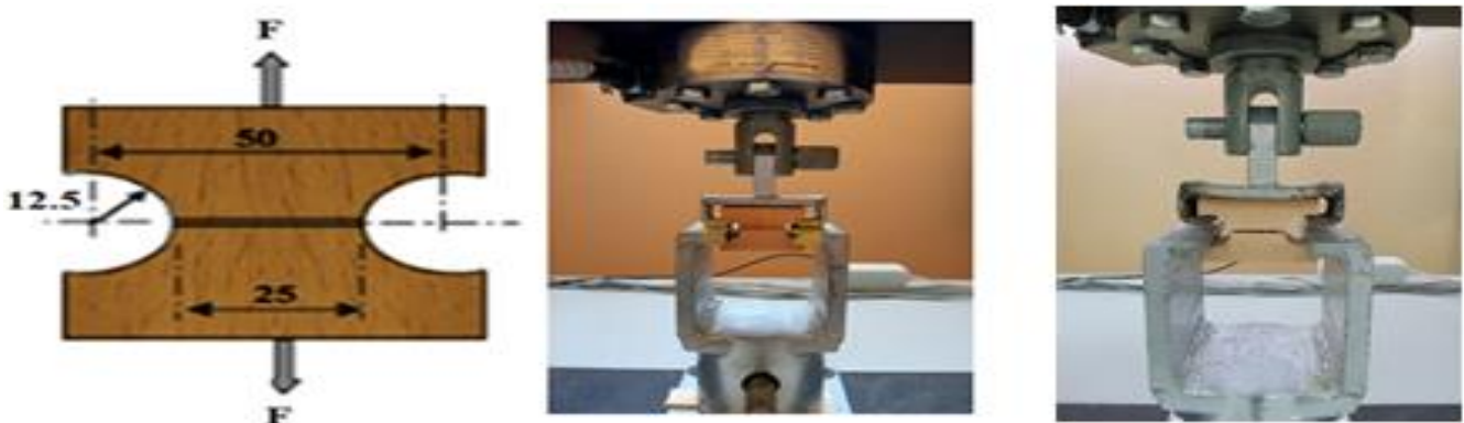
Figure 5. Apparatus used to hold specimens for the tensile strength perpendicular to fibers tests
