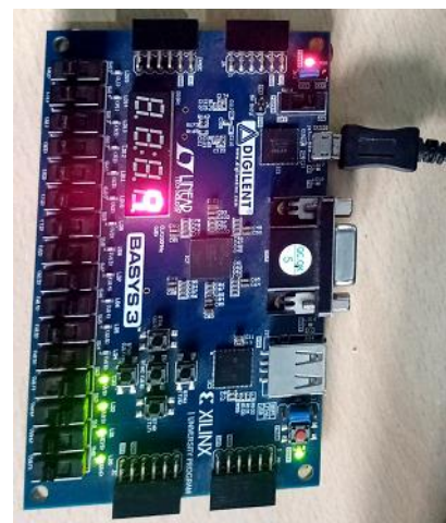
Fig.8. Representation of 2421 code for displaying hexadecimal number '9'
