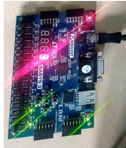
Fig.10. Representation of 5211 code for displaying hexadecimal number '3'
