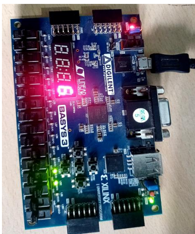
Fig.7. Representation of 2421 code for displaying hexadecimal number '6'
