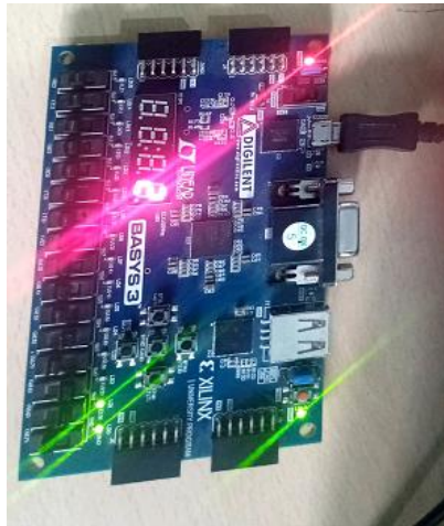
Fig.9. Representation of 5211 code for displaying hexadecimal number '2'
